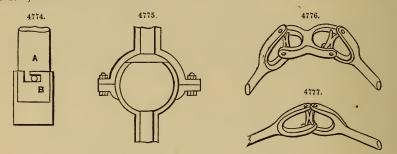
Fig. 4775, a ball-and-socket joint arranged for tubing. Figs. 4776, 4777, two kinds of universal joints.
